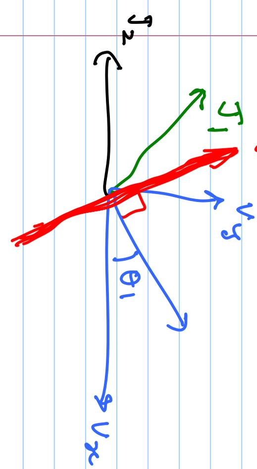
$$J_2 = L_2 \begin{pmatrix} -s_1 \\ c_1 \end{pmatrix} \quad \text{②} \quad \theta_1$$
