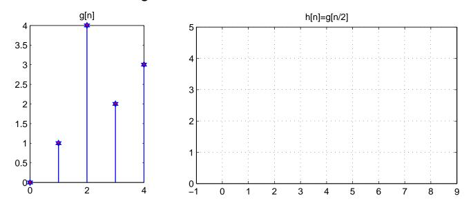
The unknown samples can be left as "undefined" or they can be interpolated, based on the the known values before and after them. (Matlab function: "interp")
