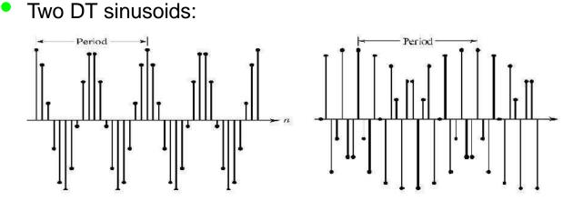
• An interesting point to note is that sometimes two DT sinusoids can be identical even if they have different Ks. For example:  $g_1[n] = \cos(\frac{2\pi}{5}n)$  and  $g_2[n] = \cos(\frac{12\pi}{5}n)$
