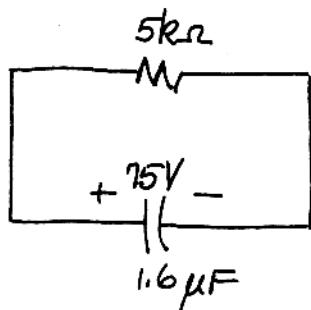
$$\begin{aligned}\tau &= 8 \times 10^{-3} = 8 \text{ ms} \\ 1/\tau &= 125 \\ i(0^+) &= \frac{75}{5} \times 10^{-3} = 15 \text{ mA} \\ i(t) &= 15e^{-125t} \text{ mA}, \quad t \geq 0^+\end{aligned}$$
