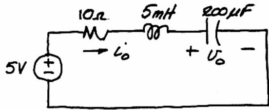
$$\alpha = \frac{R}{2L} = \frac{10}{10} \times 1000 = 1000 \text{ rad/s}; \quad \omega_o^2 = \frac{1}{LC} = \frac{(10^3)(10^6)}{(5)(200)} = 10^6$$
