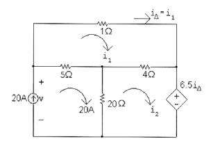
Since the bottom left mesh current value is known, we need only two mesh current equations:
