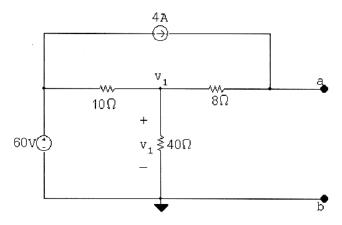
Write and solve the node voltage equation at  $v_1$ :
