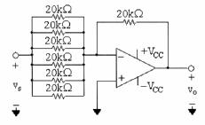
[b] To amplify a 3 V signal without saturating the op amp, the power supply voltages must be greater than or equal to the product of the input voltage and the amplifier gain. Thus, the power supplies should have a magnitude of (3)(6) = 18 V.
