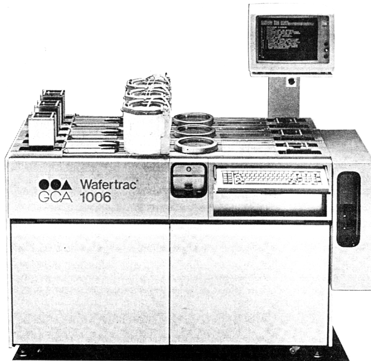
Figure 4-17 A photograph of an automated spin-coater. There are three parallel tracks for processing. At the left-hand end are three "sender" wafer cassettes, partially raised; at the right are three empty "receiver" cassettes that are lowered almost flush with the machine surface. Wafers move from left to right, through the spin and bake modules. A keyboard and CRT screen allow entry and monitoring of process variables. (Photograph courtesy of GCA Corporation, Bedford, Massachusetts. Wafertrac® is a registered trademark of GCA Corporation.)
