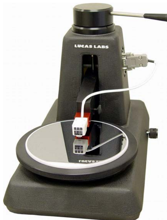
Fig. 4.17 Four-point probe with probe spacing s used for direct measurement of bulk wafer resistivity and the sheet resistance of thin diffused layers. A known current is forced through the outer probes, and the voltage developed is measured across the inner probes. (See eqs. (4.16) through (4.18).)
