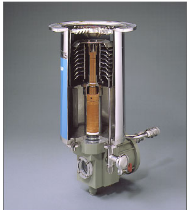
Fig. 6: Typical set-up of a two-stage refrigerator-cooled cryopump
