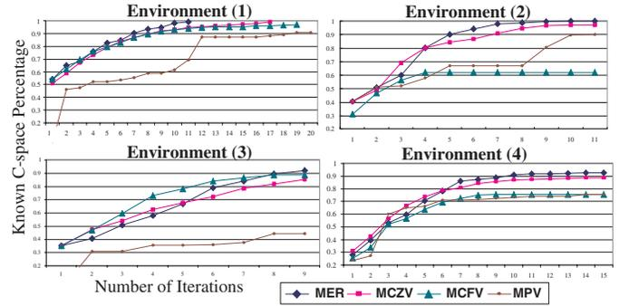
Fig. 6. Comparison of C-space exploration efficiency in environments (1), (2), (3) and (4) for the three view planning criteria: MER, MCFV and MCZV. The data shown are average performance for ten tests conducted.
