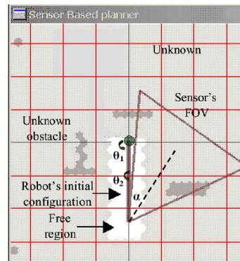
Fig. 1. Example of an eye-in-hand system: a planar 2-link robot with a triangle FOV range sensor.
