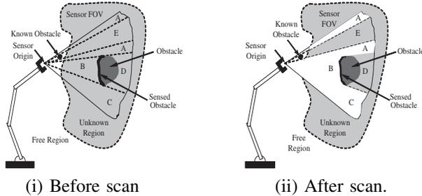
Fig. 2. A generic range sensor's FOV  $\mathcal{V}(s)$ . After this sensing action, regions A, B and C are known free, the black contour is a sensed obstacle and region D, occluded by the sensed obstacle remains unknown. Region E also remains unknown due to occlusion by an already known obstacle.
