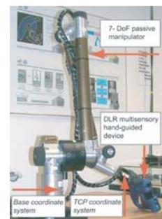
Fig. 1. Sensor principles integrated in the DLR hand-guided device
