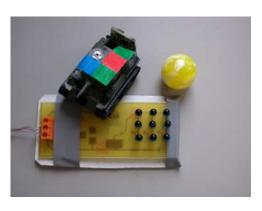
My main task was to redesign the IR communication protocol because the old one encountered some timing issues. What I need to do was program the micro-controller on the transmitter PCB to control the IR LED to generate the IR signal. The transmitter PCB was a new
