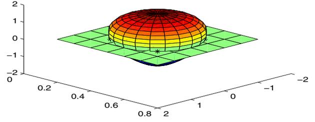
Fig. 1. The manipulated object with the 4 initial contact points (denoted by \*) in the plane  $z = 0$ . The task is a rotation around  $[1 \ 0 \ 1]^T$ . ( $z$  axis is directed upwards.)
