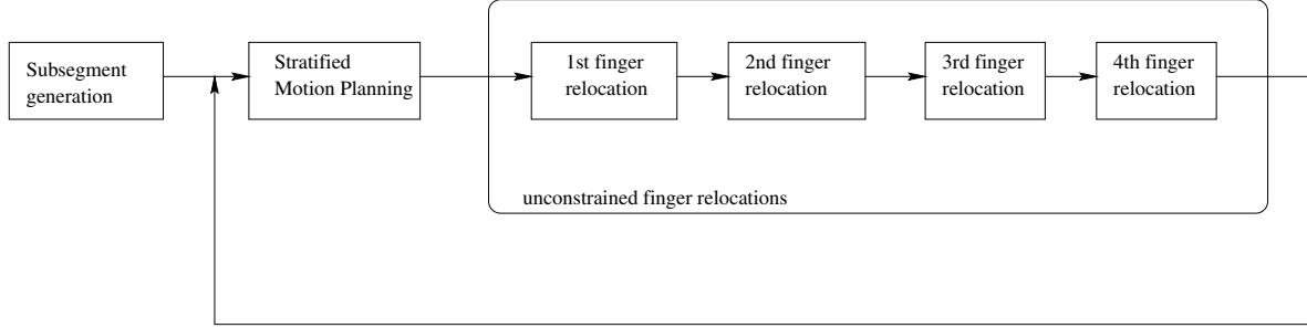
Fig. 7. The main steps of semi-stratified manipulation planning.
