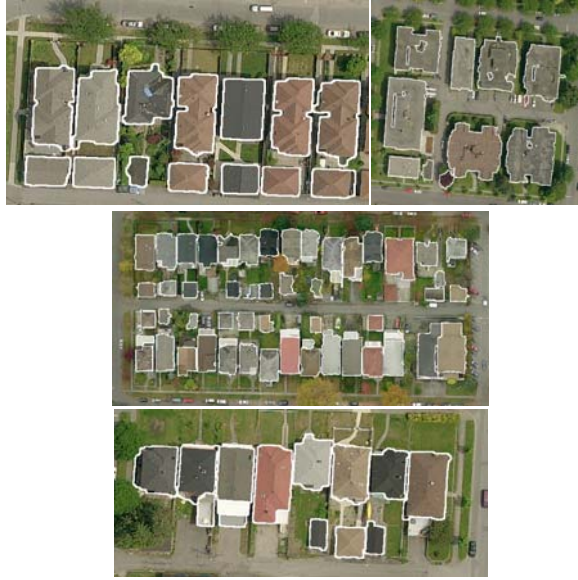
Figure 3. Extracted rooftops in 4 images.
