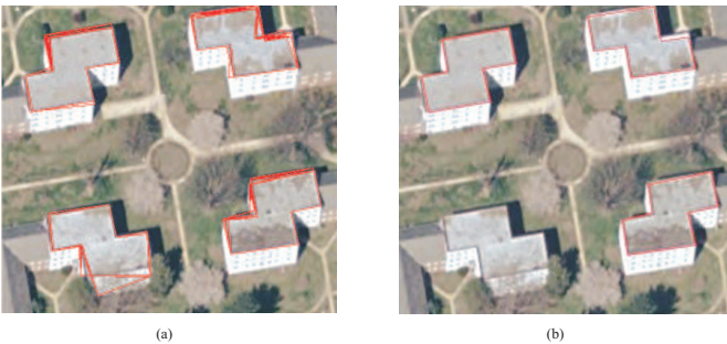
Fig. 10: (a) Rooftop hypotheses after first (a) and second (b) elimination steps for a sample scene.
