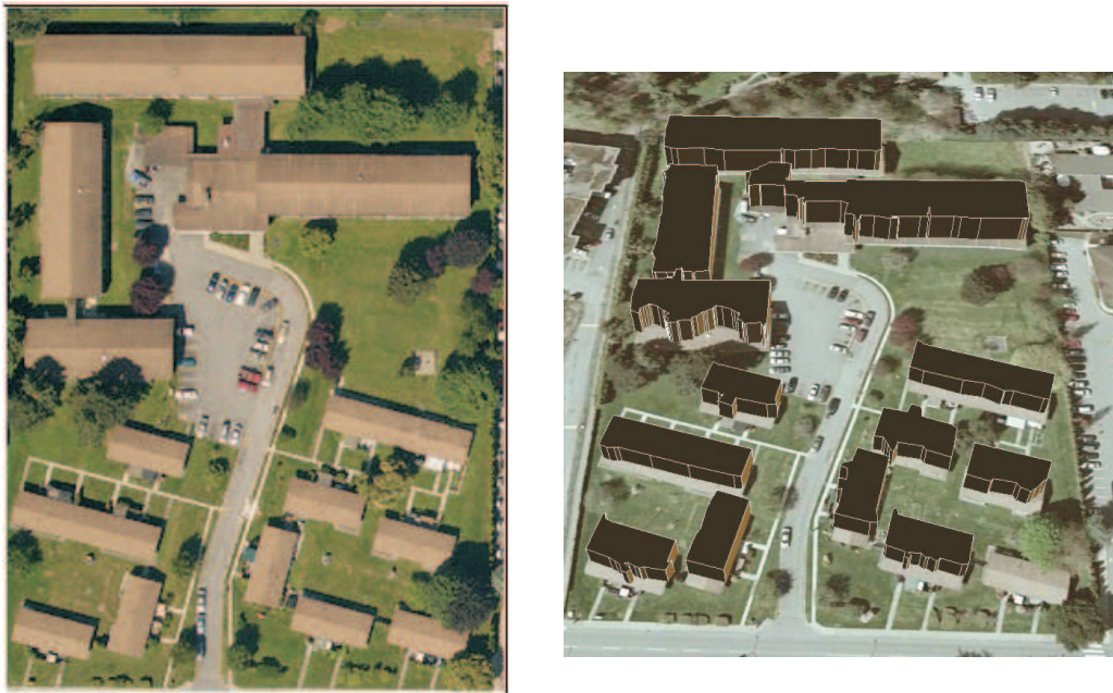
Fig. 23: Visual representation of 3D models of buildings for a sample aerial scene image reconstructed by the proposed method.
