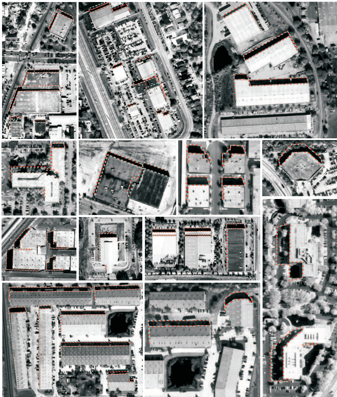
Fig. 22: Examples of the building 3D profiles of the input buildings (casted shadow footprints at the estimated height values). In these images, for each rooftop hypothesis the expected shadow footprint corresponding to the estimated height is overlaid on the ground by the red lines and the manually prepared ground truth projected shadows (corresponding to the true heights) are displayed with the blue lines.
