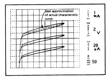
Fig. 2-23. Example of a display exhibiting looping.
