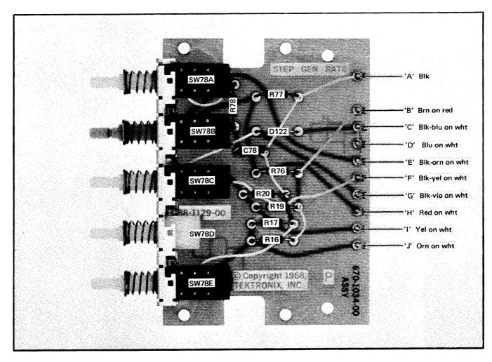
Fig. 4-11. Component locations and wiring color codes on Step Gen Rate circuit board.
