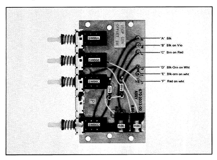
Fig. 4-9. Component locations and wiring color codes on Step Gen Offset circuit board.
