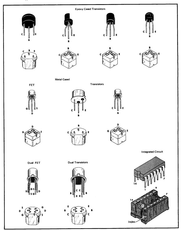
Fig. 4-2. Electrode configurations for socket-mounted semiconductor devices.
