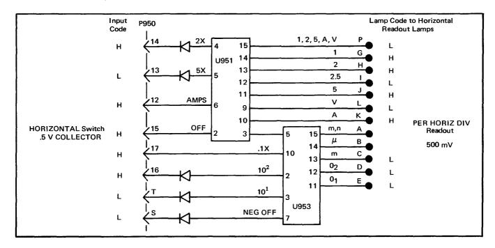
Fig. 3-13. Example of operation of Horizontal Readout decoders.
