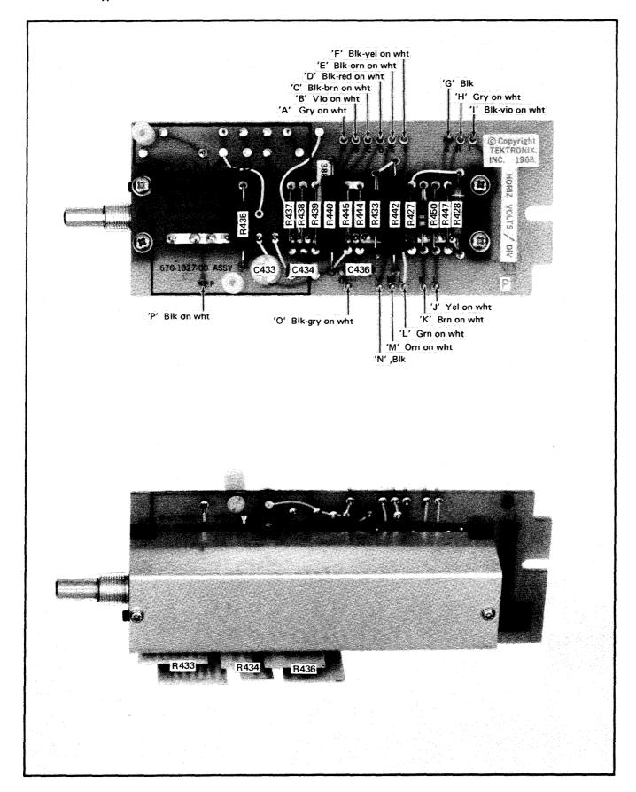
Fig. 4-13. Component locations and wiring color codes on Horiz Volts/Div circuit board.
