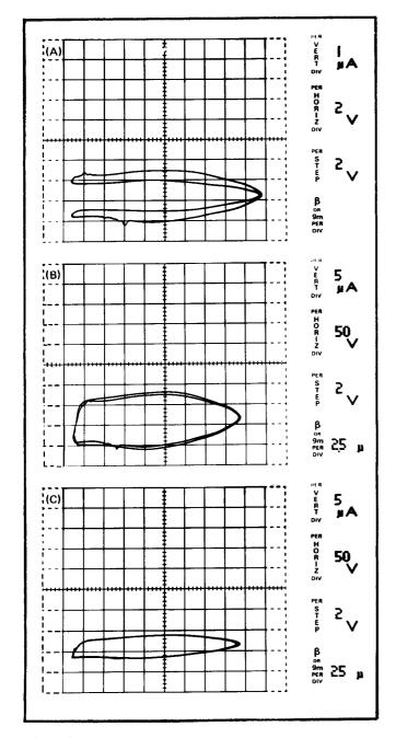
Fig. 5-12. Type 576 display of looping: (A) Display of undesirable double loop; (B) Display of uncompensated looping; (C) Display of compensated looping.
