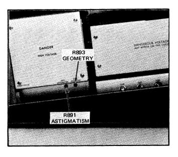
Fig. 5-4. Location of adjustments in step 4.
