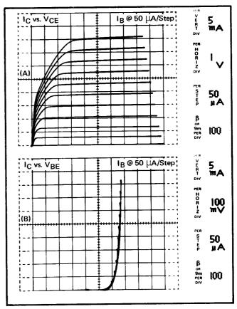
Fig. 2-13. (A) I<sub>C</sub> vs. V<sub>CE</sub> for 10 steps of base current at 50  $\mu$ A per step; (B) I<sub>C</sub> vs. V<sub>BE</sub> for 10 steps of lease current at 50  $\mu$ A per step.
