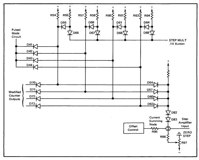
Fig. 3-6. Simplified schematic of Digital-To-Analog Converter.
