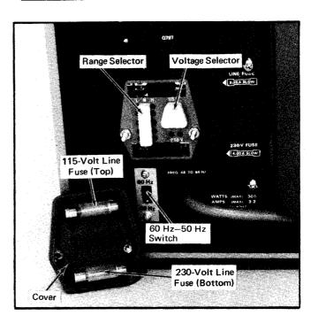
Fig. 2-1. Line Voltage Selector assembly and 60 Hz-50 Hz switch on the rear panel (shown with cover removed).
