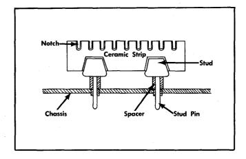
Fig. 4-4. Ceramic terminal strip assembly.
