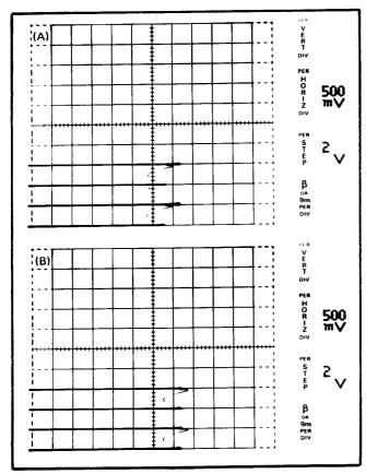
Fig. 5-10. Type 576 display of Collector Supply peaks for adjusting DELAY adjustment R24: (A) incorrect adjustment; (B) correct adjustment.
