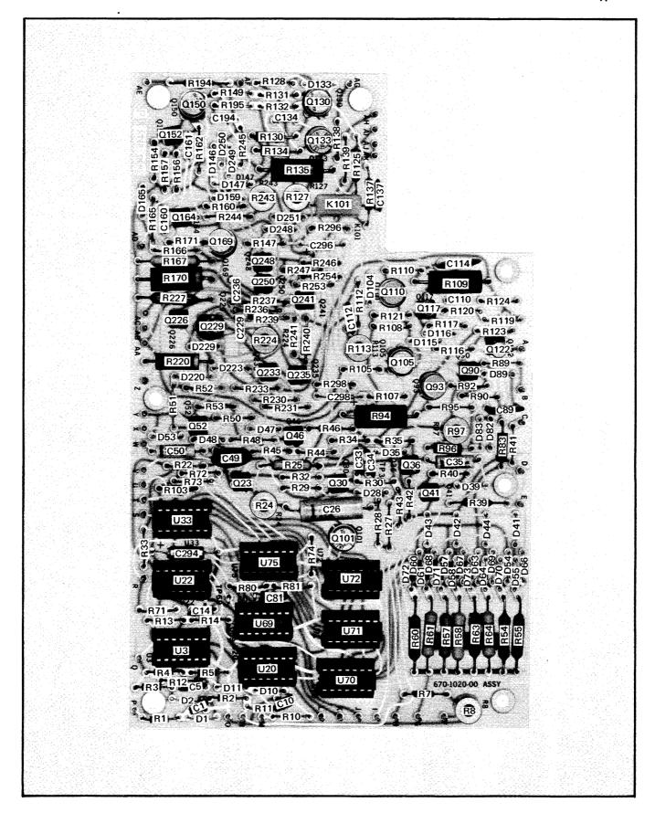
Fig. 4-6. Component locations on Step Gen circuit board.
