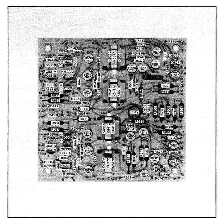
Fig. 4-16. Component locations on Display Amp circuit board.
