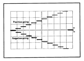
Fig. 2-24. Step Generator output in both polarities
