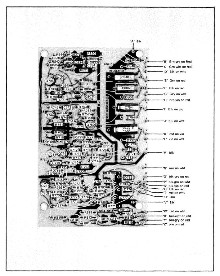
Fig. 4-24. Component locations and wiring color codes on L. V. Regulator circuit board.
