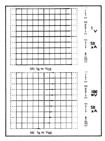
Fig. 2-14. (A)  $I_B$  vs.  $V_{CE},\,I_b$  @ 50  $\mu\!A$  per division; (B)  $I_B$  vs.  $V_{BE},\,I_R$  @ 50  $\mu\!A$  per division.
