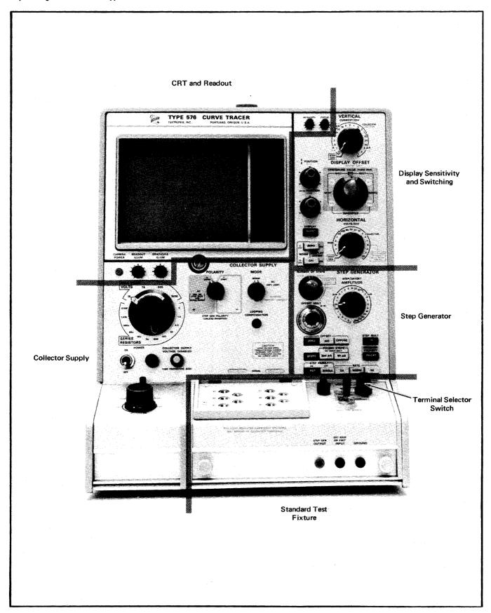
Fig. 2-2. Front-panel controls, connectors and readout.
