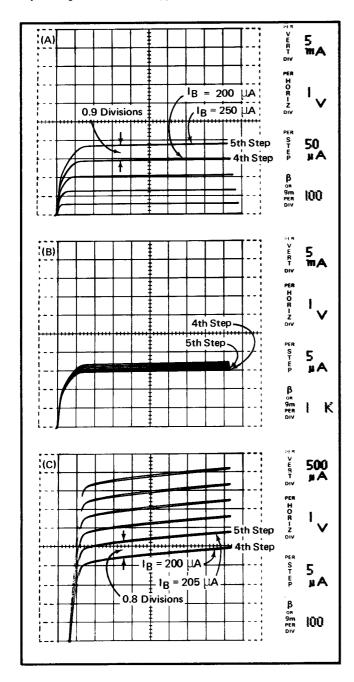
Fig. 2-18. Measurement of  $\beta$  of transistor, (A) Coarse measurement; (B) Offsetting of display and .1X multiplication of step amplitude; (C) 10X magnification of vertical display.
