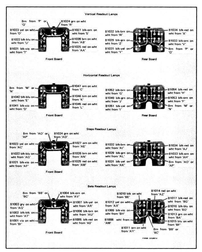
Fig. 4-22. Component locations and wiring color codes on Readout Lamp circuit boards.
