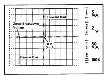
Fig. 2-10. Display of Zener diode I vs. V characteristic with PO-LARITY switch set to AC.
