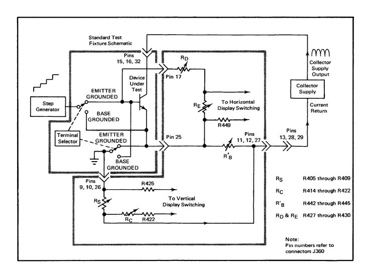
Fig. 3-9. Simplified schematic of Display Sensitivity Switching and Standard Test Fixture schematics for measurement of collector current (I<sub>C</sub>) and base-emitter voltage (V<sub>BE</sub>) on emitter-base voltage (V<sub>EB</sub>).
