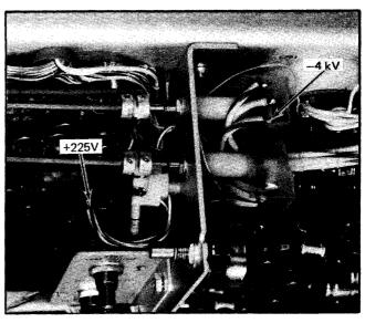
Fig. 5-3. Location of high voltage test points on right side of instrument.
