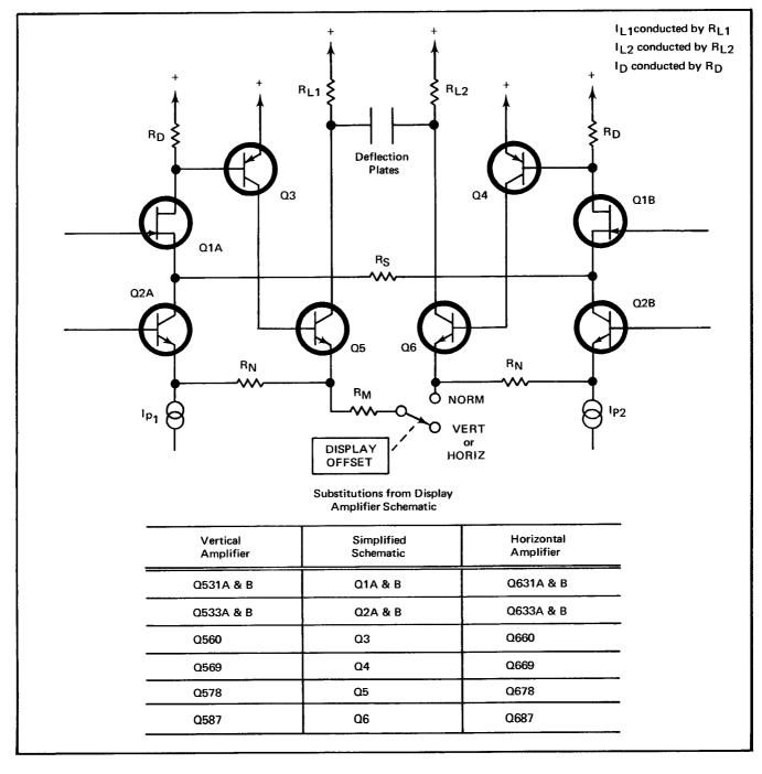
Fig. 3-12. Simplified schematic of display amplifier.
