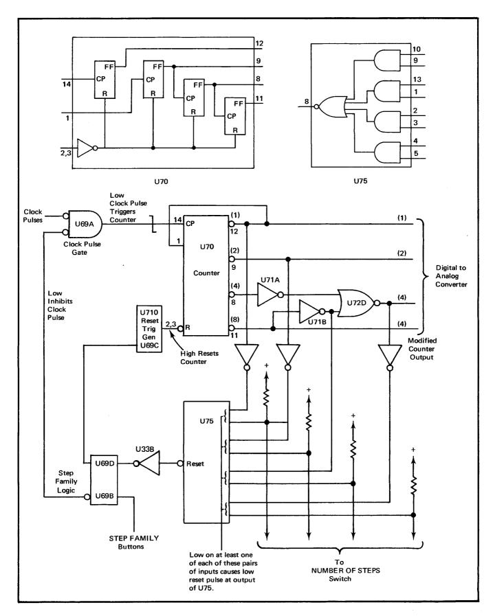
Fig. 3-5. Block diagram of counter and reset logic.
