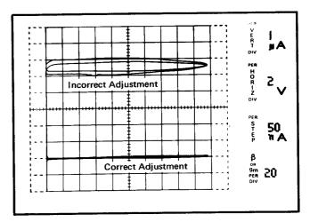
Fig. 2-9. Adjustment of LOOPING COMPENSATION control.
