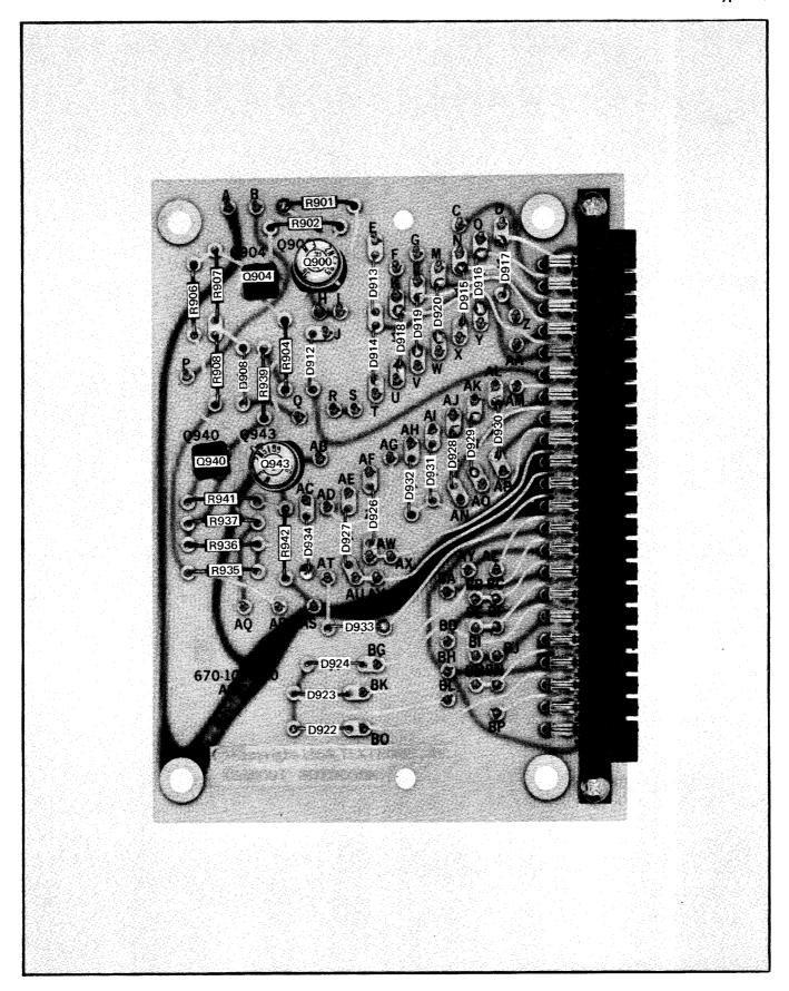
Fig. 4-18. Component locations on Readout Interconn circuit board.
