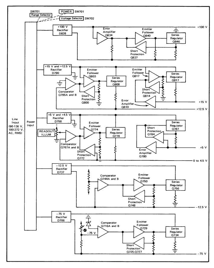
Fig. 3-14. Block diagram of L. V. Power Supply.
