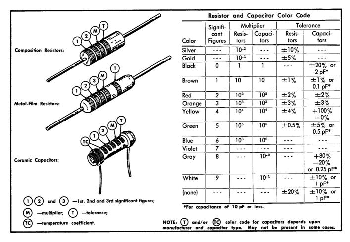
Fig. 4-1. Color-code for resistors and ceramic capacitors.
