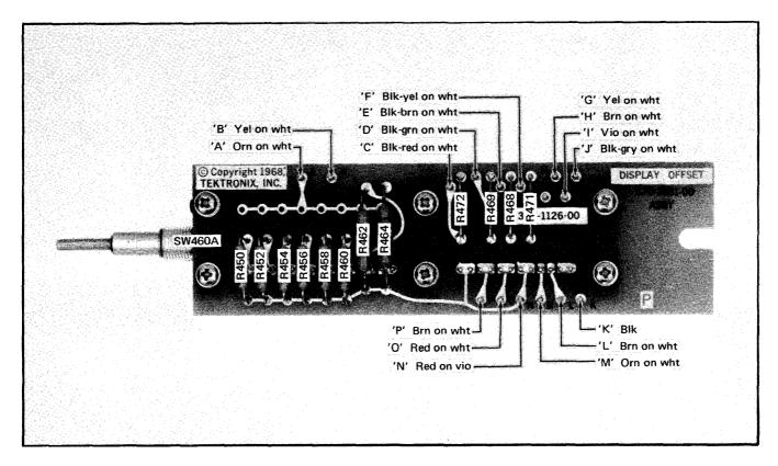
Fig. 4-15. Component locations and wiring color codes on Display Offset circuit board.
