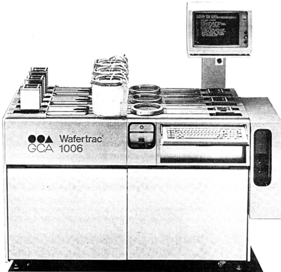
Figure 4-17 A photograph of an automated spin-coater. There are three parallel tracks for processing. At the left-hand end are three "sender" wafer cassettes, partially raised; at the right are three empty "receiver" cassettes that are lowered almost flush with the machine surface. Wafers move from left to right, through the spin and bake modules. A keyboard and CRT screen allow entry and monitoring of process variables. (Photograph courtesy of GCA Corporation, Bedford, Massachusetts. Wafertrac® is a registered trademark of GCA Corporation.)
