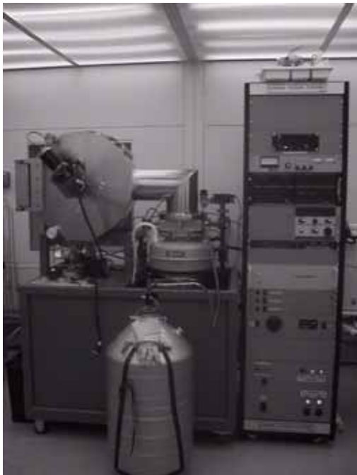
Figure 12-24 Photograph and schematic of a commercial sputtering system used for silicon IC fabrication (courtesy Balzers).
