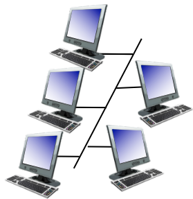
shared wire (e.g., cabled Ethernet)
