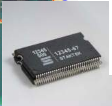
Package-on-Package (POP) 3D stacking
