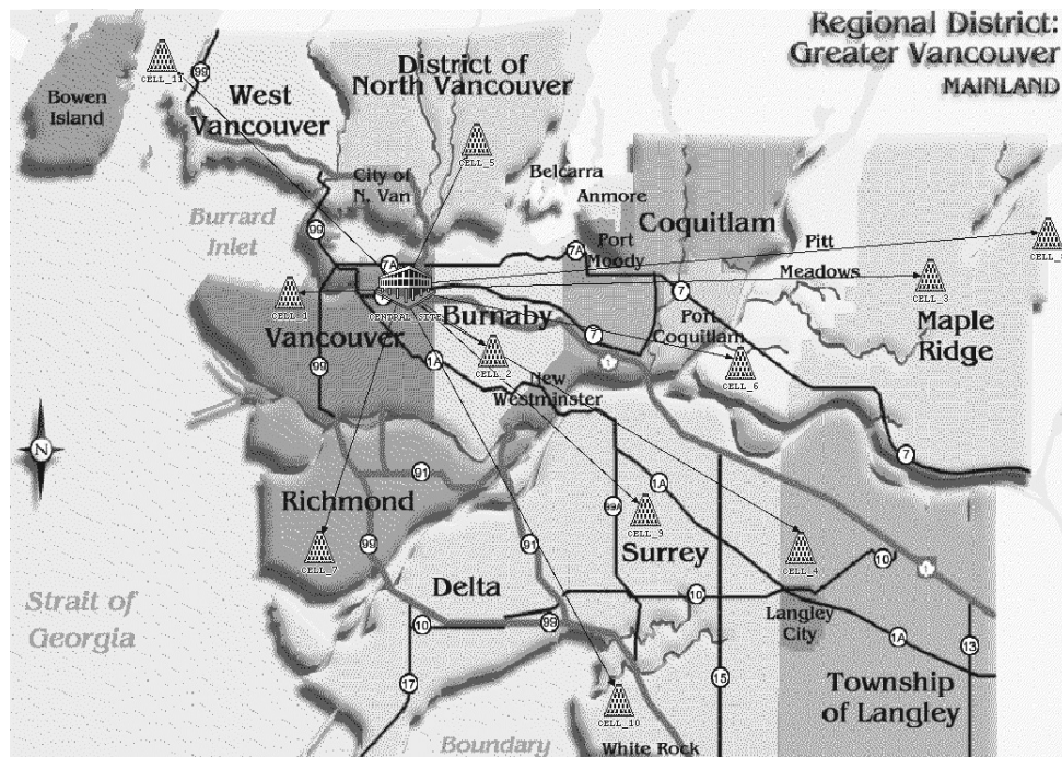
Figure 4. OPNET model of the E-Comm network. The network model consists of a central site located in East Vancouver and 11 cells covering various municipalities of the Greater Vancouver Regional District. The cells are connected to the central site via point-to-point links.
