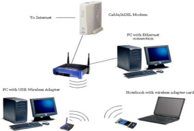
Figure 3: WiFi client/station connection [5].
