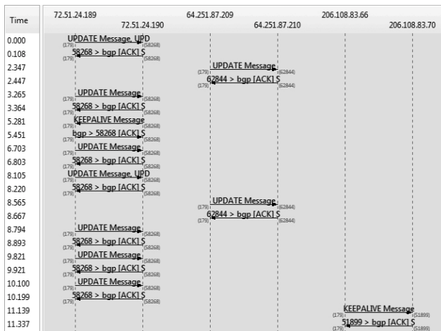
Figure 9. Flow graph of collected traffic. Shown are time stamps of correspondence between BGP peer routers.
