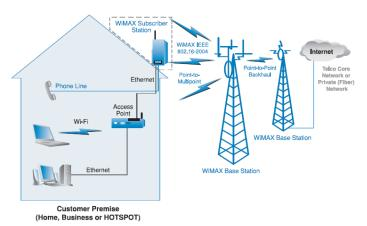
Figure 6. WiMAX client station connection.
