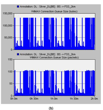
Figure 16. Downlink performance: (a) 2 km station received and lost packets/sec and (b) base station downlink queue.
