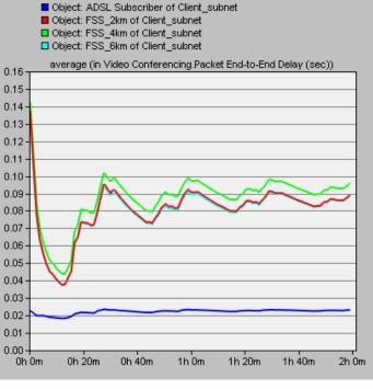
Figure 17. End-to-end packet delay: (a) average and (b) instantaneous values.
