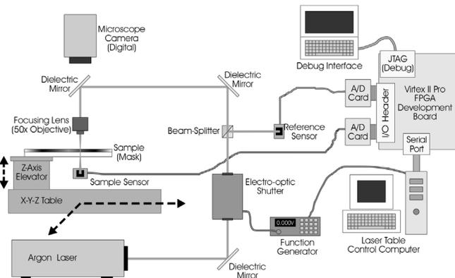
Figure 3. Laser-based Transparency Meter System.
