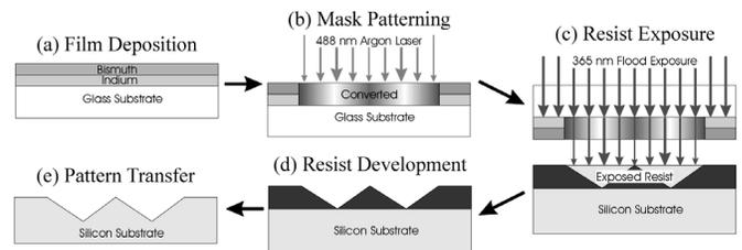
Figure 1. Creation and use of a bimetallic grayscale mask: (a) bimetallic film deposition, (b) laser exposure to create transparent oxide, (c) usage of the mask to limit photoresist exposure, (d) removal of exposed resist via development, and (e) resulting 3D-structure after pattern transference.
