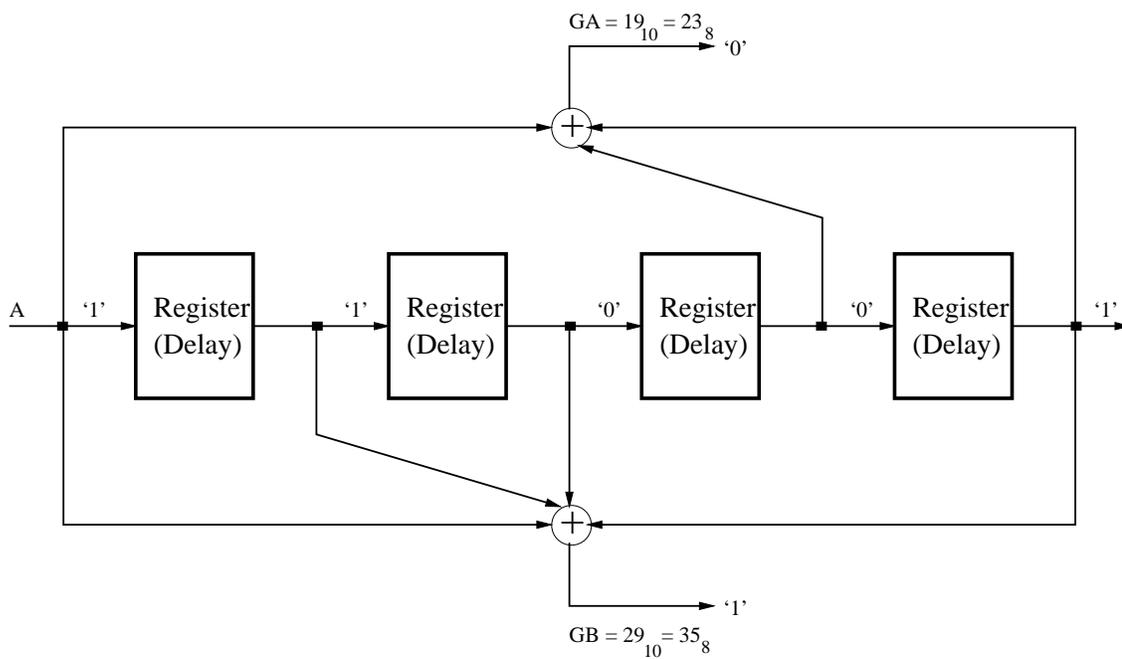
Figure 3.6: Block diagram of the encoding circuit illustrating functionality.
