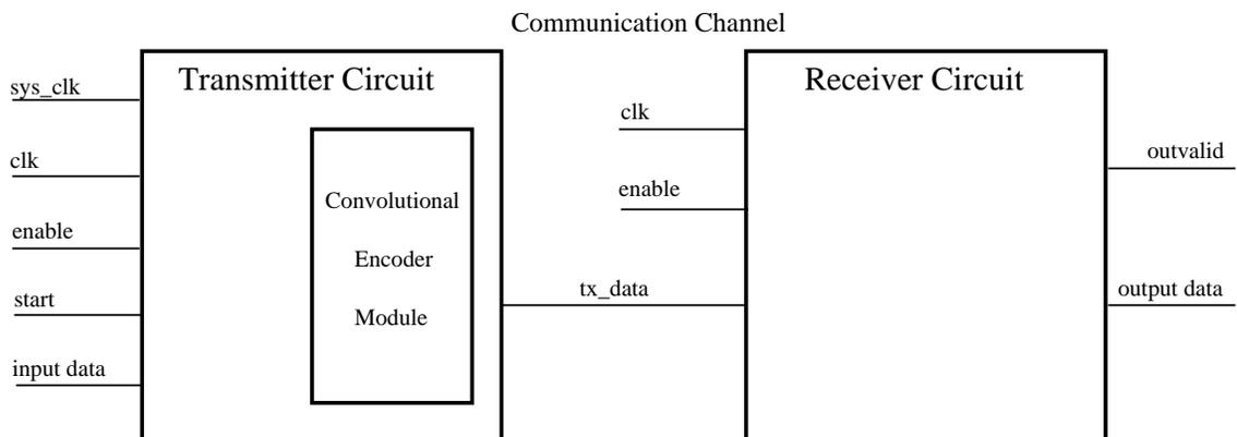
Figure 3.1: Block diagram of the transmitter-receiver system highlighting the convolutional encoder.
