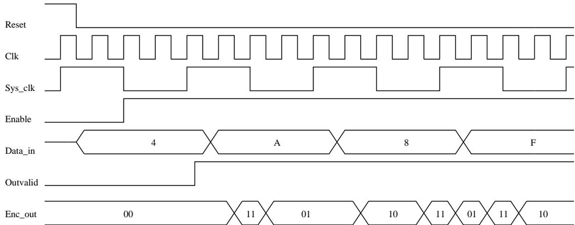
Figure 3.7: Timing diagram of the convolutional encoder.
