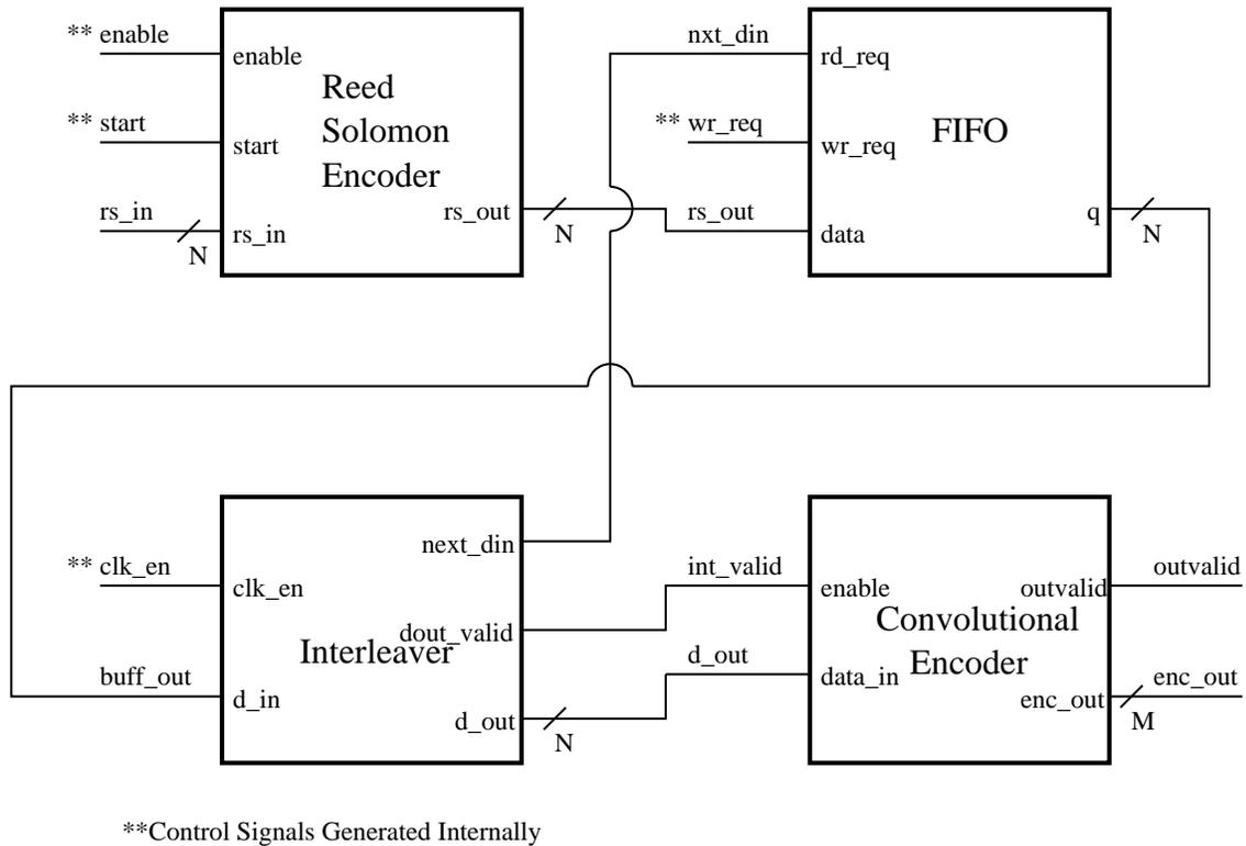
Figure 3.4: The actual transmitter block diagram implemented with cores.
