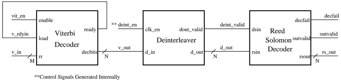
Figure 3.8: The ideal receiver block diagram implemented with cores.
