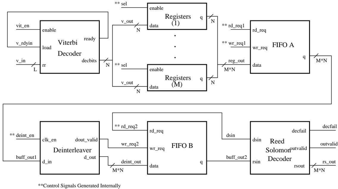
Figure 3.9: The actual receiver block diagram implemented with cores.
