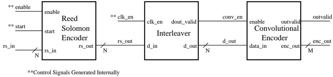
Figure 3.2: The ideal transmitter block diagram implemented with cores.
