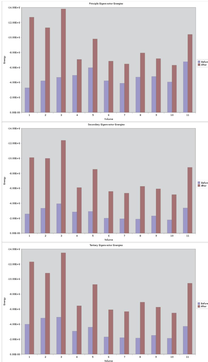
**Figure 5.** Whole 3D volume energy  $E = \sum_{x \in \Omega} E(e_i, x)$  before and after re-alignment for 11 available heart datasets. The bar plots above show that there is a decrease in energy after the re-alignment procedure indicating equilibration to a more spatially smooth eigenvector field. Note that this re-alignment only reverses the direction of the eigenvector where needed with a sign change  $e_i \mapsto -e_i$ , and does not change the original orientation of the vectors in space.
