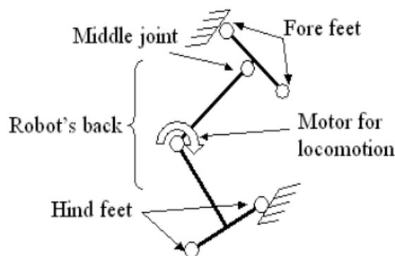
Figure 5: Proposed Operation of a simple gecko-inspired climber [6]
