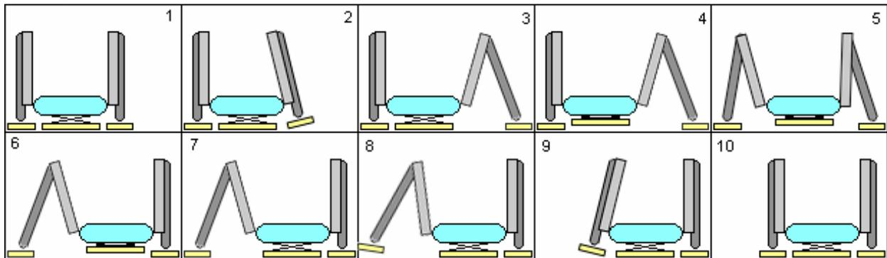
**Inside Corner Transition:**
