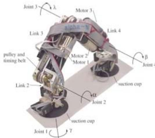
Figure 2. The Under Actuated Climber, University of Utah [3]
