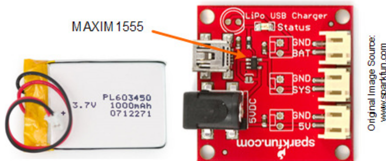
Figure 8: Li-Ion Battery and Maxim1555 Charge Board. [22] [23]
