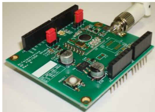
Figure 16: Arduino RF Transceiver Shield
