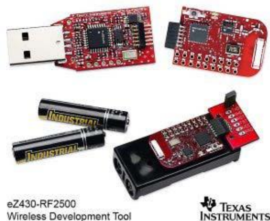
Figure 14 – Picture of ez430-RF2500 Development Kit
