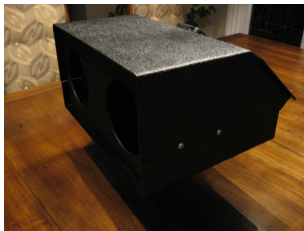
Figure 22: Assembled prototype case for portable radar system; note that the handle is not shown in this image
