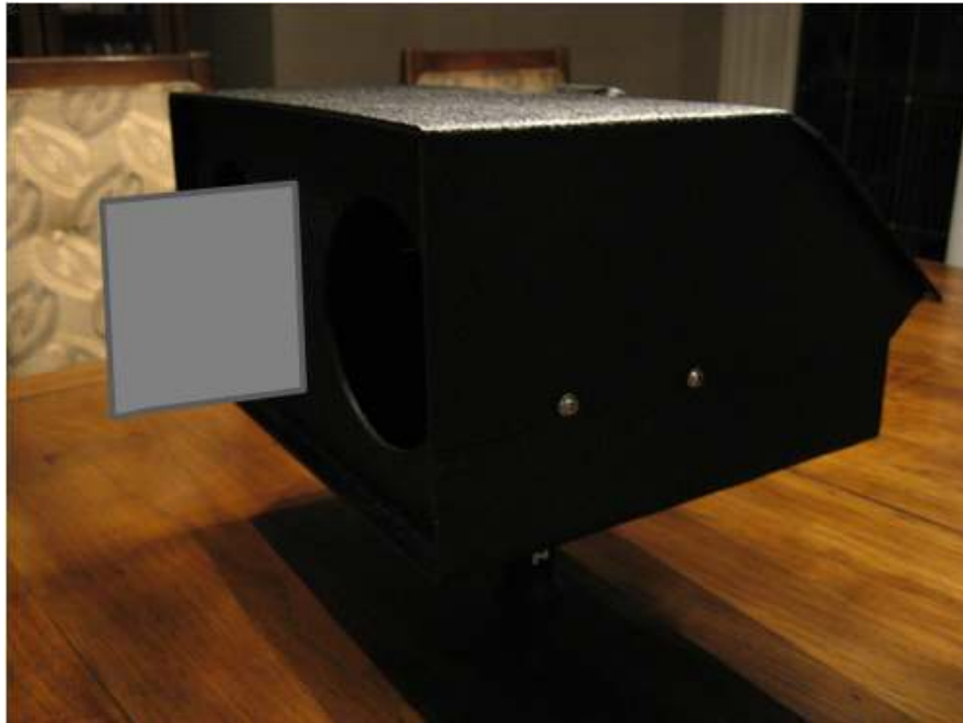
Figure 25: Physical barrier designed to limit the amount of internal noise between the two antennas
