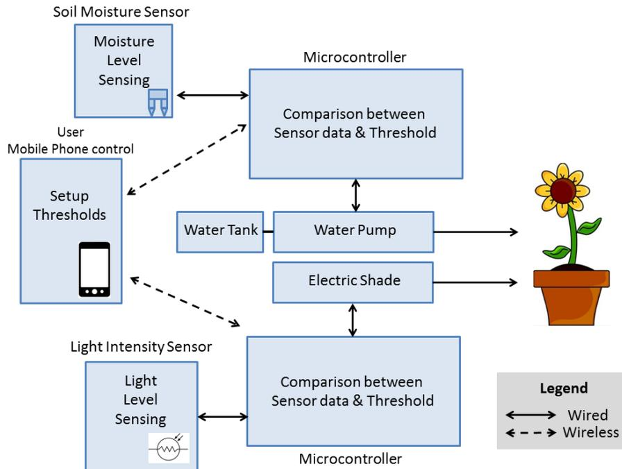
**Figure 1: Smart Planting System High-level Block Diagram**
