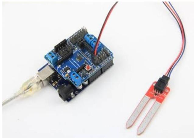
Figure 2: Soil Moisture Sensor Compatible with Microcontroller
