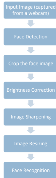
FIGURE 23 GENERAL STEPS FOR FACE RECOGNITION INCLUDING PRE-IMAGE PROCESSING FILTERS TO IMPROVE THE FACE RECOGNITION ACCURACY
