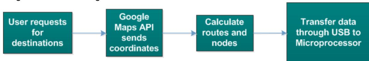
**Figure 2-2: NaviCane's Software Application Process Flow Diagram**
