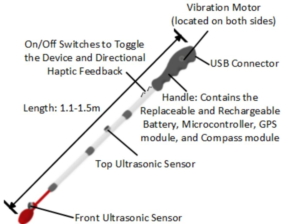
**Figure 2-4: NaviCane's Mechanical Enclosure**
