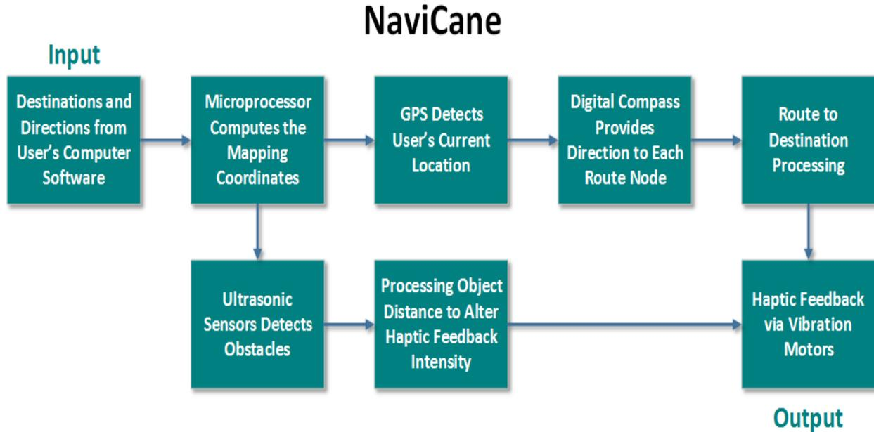
Figure 2-3: NaviCane's Top-Level Block Diagram
