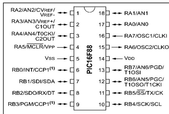
FIGURE 9 PIC16F88 CONFIGURATION [6]
