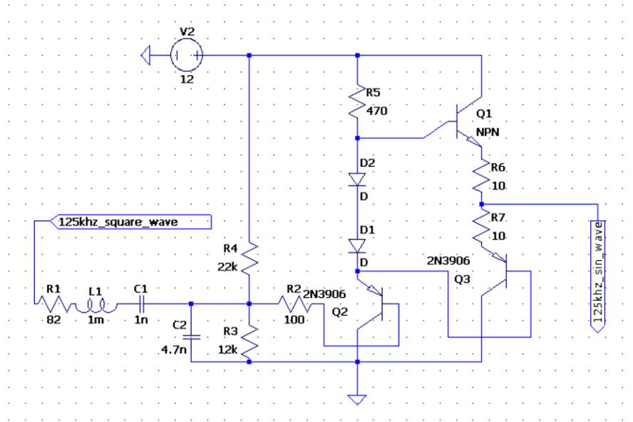
FIGURE 6 SCHEMATIC OF POWER AMPLIFIER AND ANTENNA
