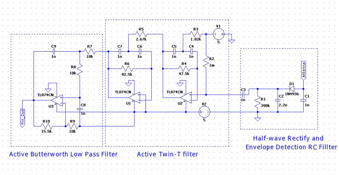
FIGURE 8 ENVELOPE DETECTOR AND FILTERS
