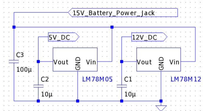
FIGURE 3 POWER SUPPLY CIRCUIT
