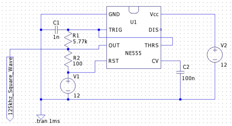
FIGURE 5 CARRIER FREQUENCY CLOCK GENERATOR
