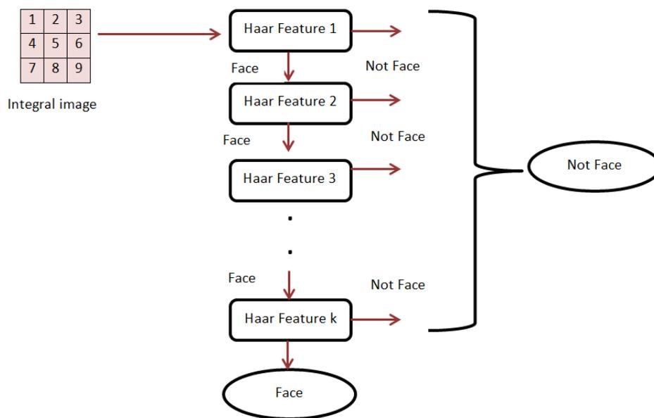
FIGURE 13 FACE DETECTION ADABOOST FILTER
