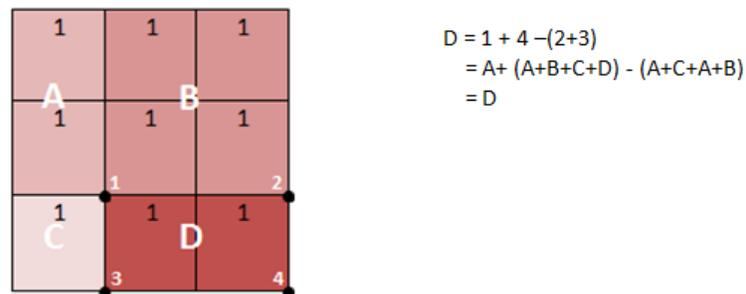
FIGURE 12 INTEGRAL IMAGE CALCULATION
