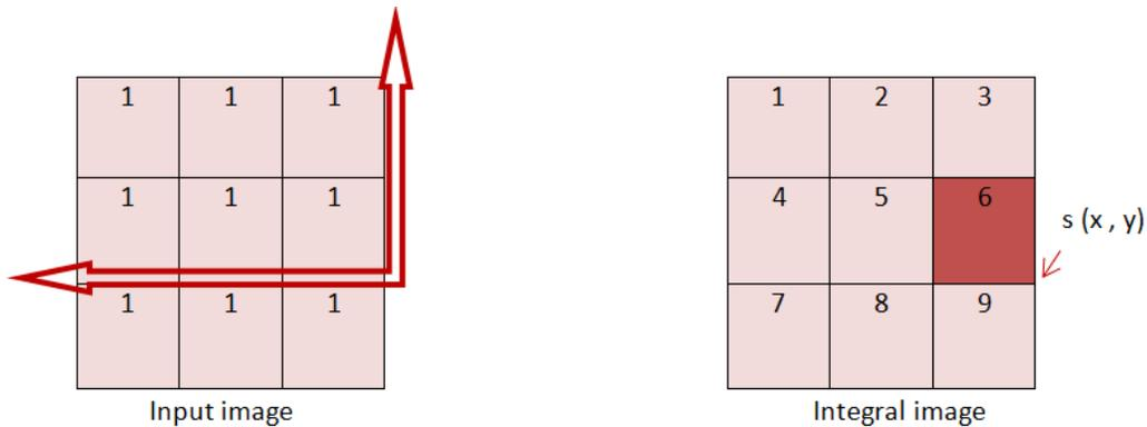
FIGURE 11 INPUT-INTEGRAL IMAGE ILLUSTRATION
