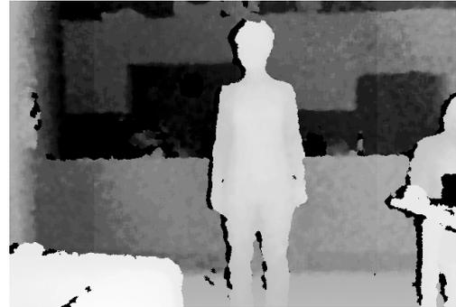
Figure 11 Sample Depth Image Captured by Kinect Depth Camera
