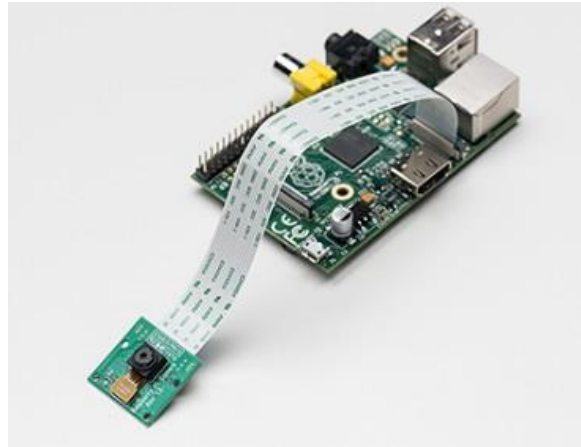
Figure 16: Raspberry Pi camera connected to the board
