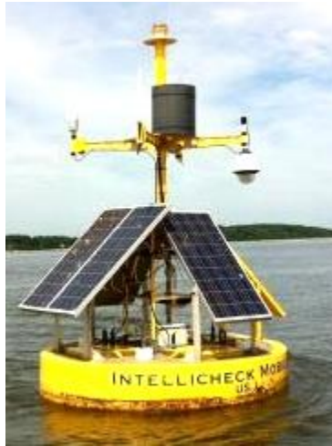
Figure 1: Solar-Powered Navigational Buoy [5]
