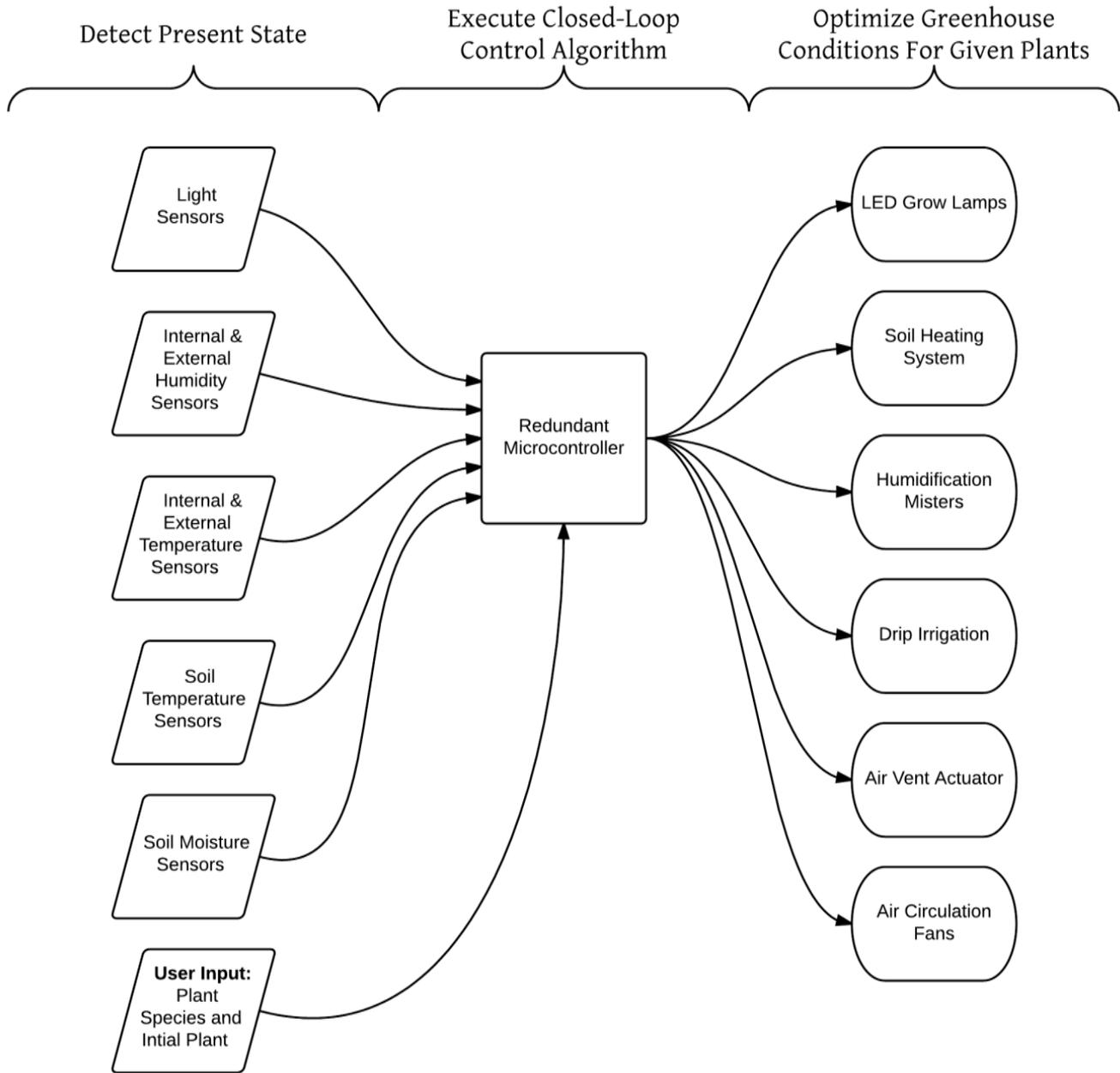
Figure 1 - Inputs, Control, and Outputs of Automation System
