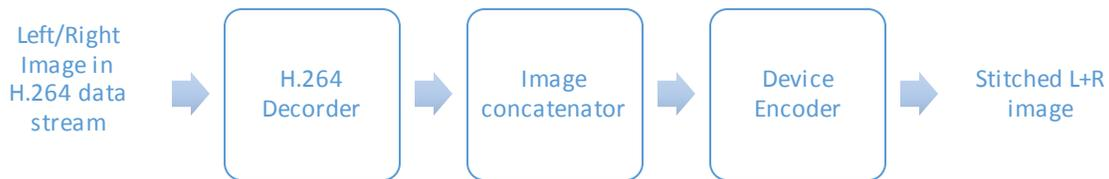
**Figure 17: Block diagram for Image data transfer**
