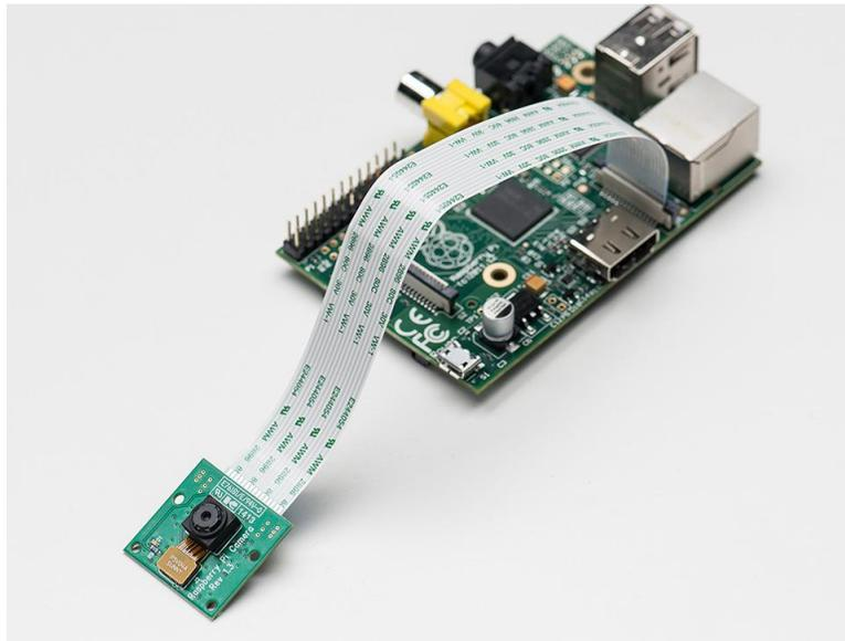
**Figure 5: RPi Camera Module Board connected to a RPi (B-Model) via a CSI cable [5]**
