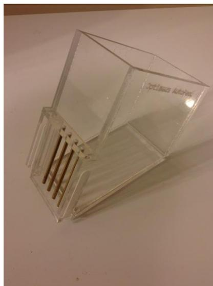
Figure 6: Hopper assembly after laser cutting
