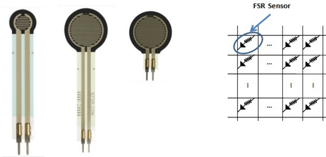
Figure 2: FSR sensor series and model of FSR matrix array
