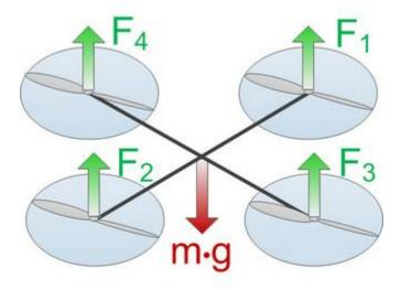
**Figure 7:** Balance of forces due to the motors and gravity. [5]
