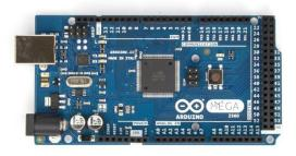
Figure 5: The Arduino Mega 2560. [10]
