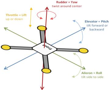
Figure 3: Angles of rotation of quadcopter. [4]
