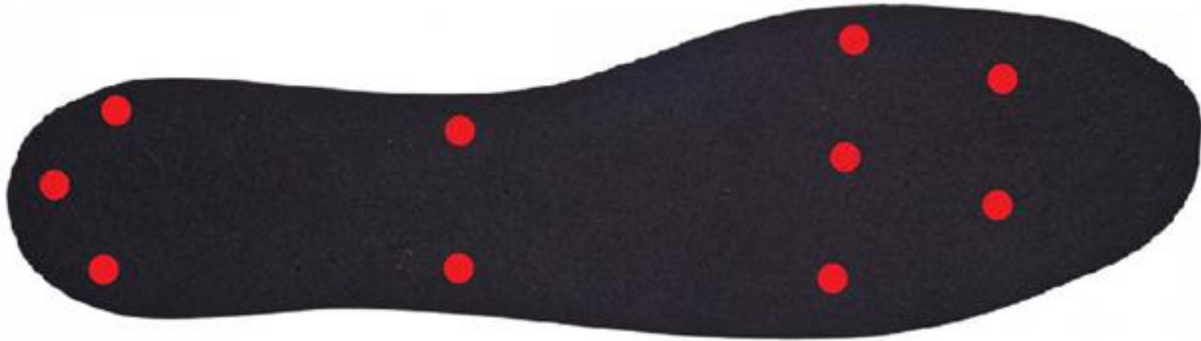
Figure 5: 10 Force Sensitive Resistors on the Insole
