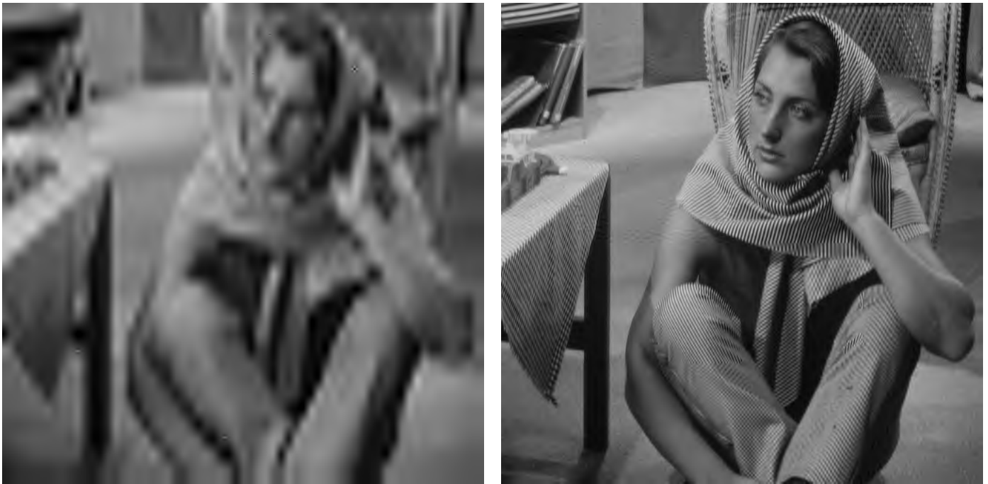
Fig. 4. Barbara image transmitted through a channel with 10% loss rate, before JSCD on left (PSNR = 22dB) and after JSCD on right (PSNR = 28.9dB)
