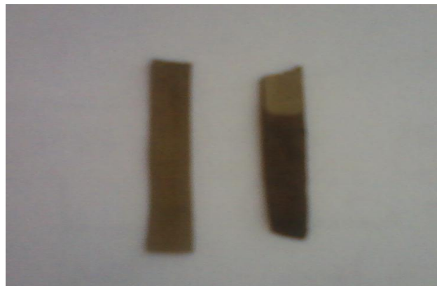
Fig. 4. A piece of C-NCPs before Chloridation (Right), and chloridized electrode (Left).
