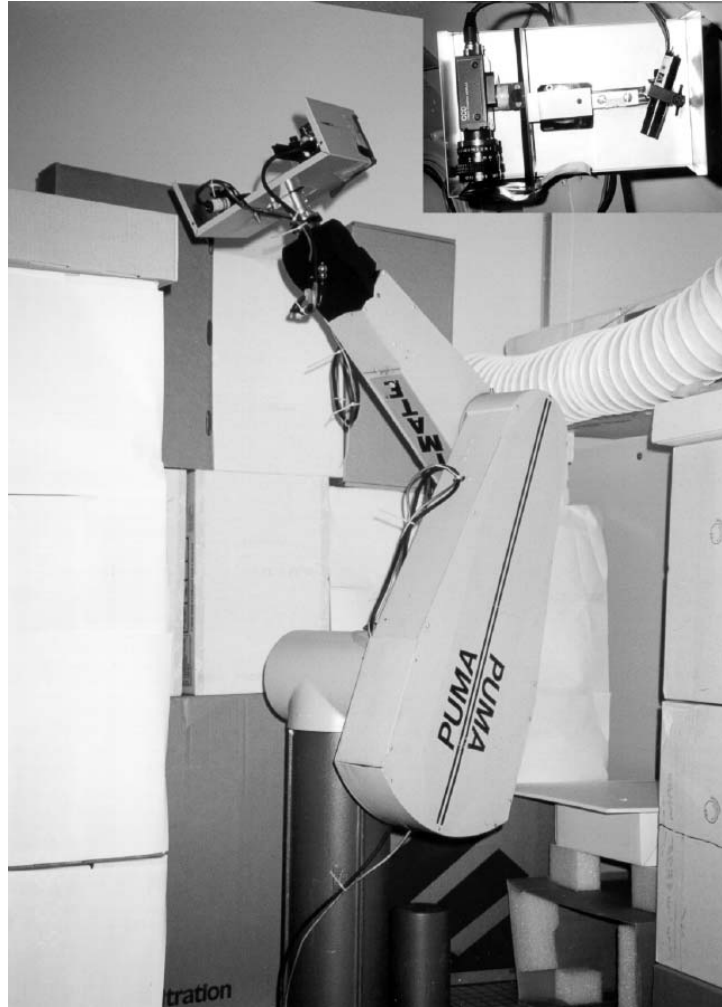
Figure 1.3: The experimental testbed for sensor-based MP. The robot is a PUMA 560 with 6 degrees of freedom. The “eye” sensor, a triangulation based area scan laser range finder, is mounted on the PUMA wrist. The inset shows an enlarged view of the sensor with the camera on the left and the laser stripier on the right. The sensor gives distances of the objects (within a certain field of view and range) from the sensor.
