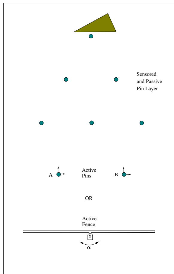
Figure 6-3 Notion of proposed dynamic environment setup. The first layer consists of passive pins with sensors while the second layer may consist of a layer of active pins (moving and/or retractable) or an active fence to orient the part after data is gathered in the first layer.
