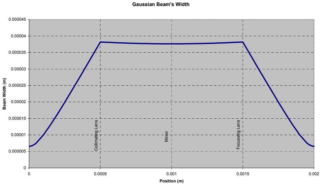
Figure 49: Plot of Gaussian beam's radius vs. position in optical switch.
