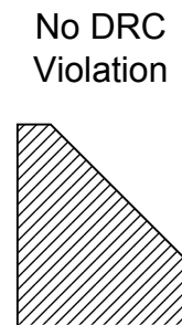
Figure 61: Acute angle has been chopped to avoid DRC error.
